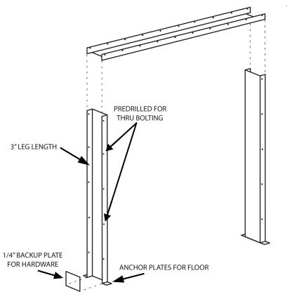
Hinge locations are reinforced with 1/4" steel plate.
